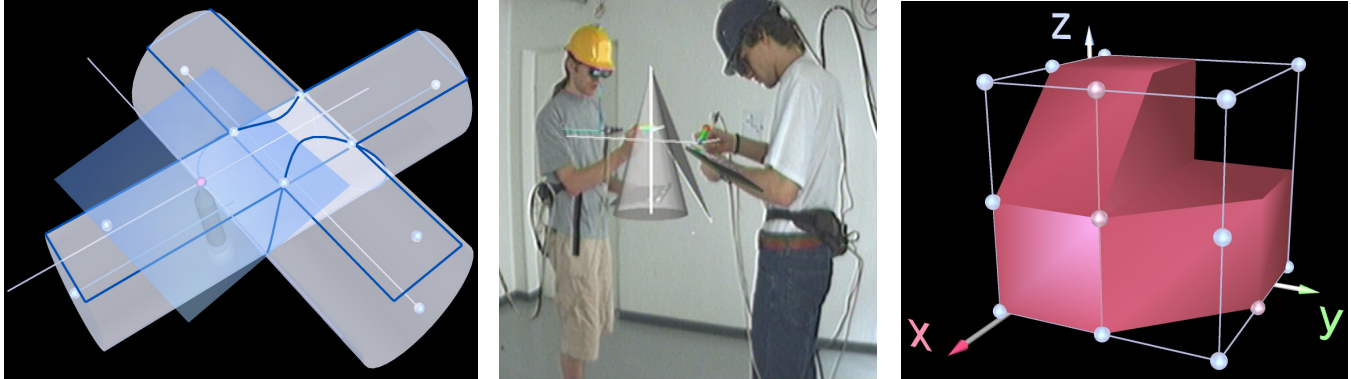
Figure 1: Geometric constructions done with Construct3D (left: 2 nd order intersection curve, right: Tschupik cube demonstrating basic Boolean operations on solids). Collaborative work in Construct3D (middle).
