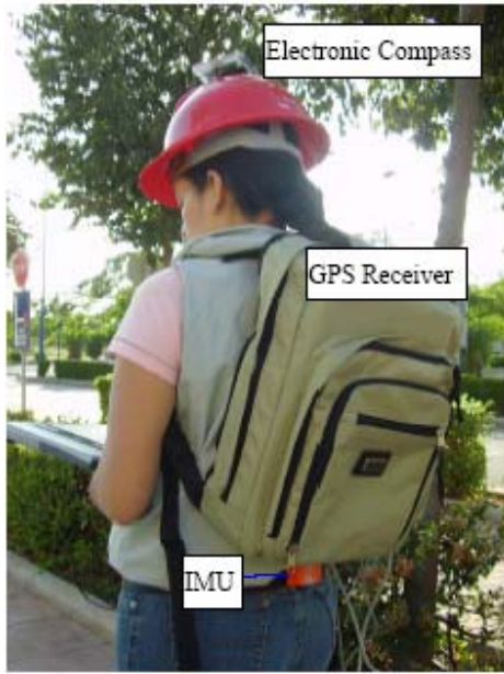
Figure1. Setup of the personal positioning system.
