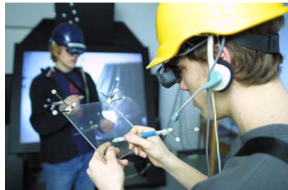
Figure 2: Two students collaborate in our standard lab setup, wearing an HMD, holding a wireless pen and panel. All devices are optically tracked.
