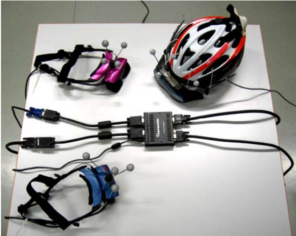
Figure 2: One input and 3 output connectors. Three HMDs (two Emagin Z800 and one Sony Glasstron) are attached to the Matrox TripleHead2Go. In our 6-user setup three more Sony Glasstron HMDs were attached to another TripleHead2Go box.
