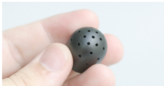
(b) CNC-machined sample from the initial production run.
