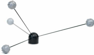
(b) Assembled four-marker rigid-body target.
