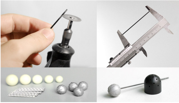
(a) We are using a Dremel rotary tool with an attached diamond cut-off disc to cleanly trim our solid carbon-fiber rods. All rod lengths are verified with a sliding caliper to within \pm 0.5 mm.
