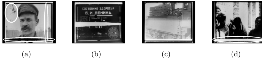
Fig. 1. Artifacts often found in archive film. Figure 1(a) shows a frame with several artifacts: dirt (top left), vertical scratch (right), frameline copied into the image (bottom). The frame in Figure 1(a) has a tear in the middle. Errors introduced during copying include unwanted changes in intensity and contrast as well as visible framelines depicted in Figures 1(c) and 1(d), respectively.
