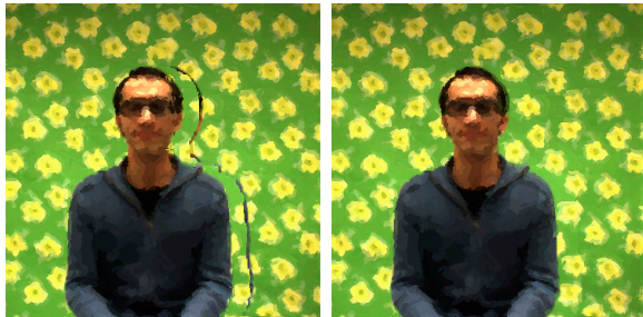
Figure 8: Final painting of right view. On the left, painting generated without dilation of the occlusion map (visible seam due to depth map inaccuracies). On the right, painting generated after dilation of the occlusion map (no seams visible, depth inaccuracies compensated).
