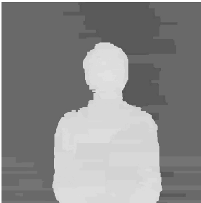
Figure 4: Depth map in the geometry of the left view. Missing values reconstructed from neighboring values.
