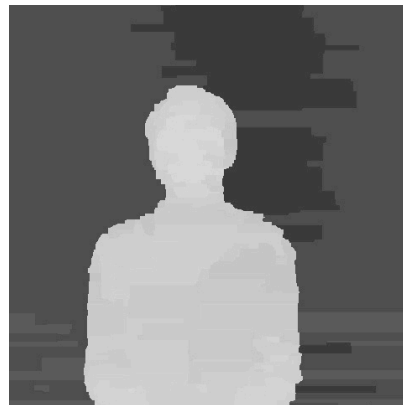
Figure 5: Depth map in the geometry of the right view. Missing values reconstructed from neighboring values.
