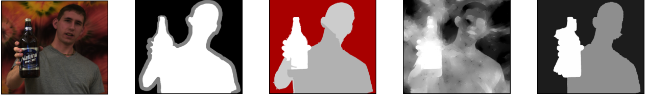
(a) Input image taken from [13] (b) User defined trimap (c) Our defocus map using (b) (d) Defocus map of [1] (e) Depth map of [13] Figure 6. A loose comparison of different defocus estimation methods. Our defocus map (c) was generated with the user-defined trimap (b). The methods of [1, 13] (d,e) are automatic. Here, white encodes small defocus/depth, black means large defocus/depth, and red means background region which is not estimated by our approach. Note, that our result is much cleaner than that of [1] (d) and is of comparable quality to [13] (e). It is important to note that [13] requires the image to be captured with a specialized aperture as well as an exact calibration of the PSF at several depths. Also our solution was computed in a few seconds, thus is orders of magnitudes faster than [13].
