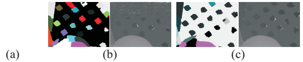
Figure 3. MDL prior. (a) Crop of the Cones image. (b) Results without using our MDL prior. Surface labels are shown left and disparity results are shown right. The background is modeled by a large set of different surfaces. (c) Results using our MDL prior. Large parts of the background are modeled by the same surface.
