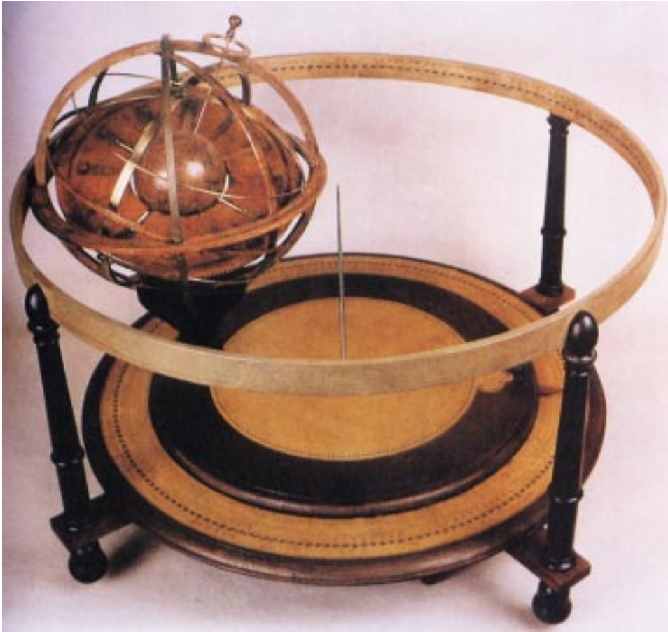
Figure 2.2: Early Copernican Tellurium, completed around 1634 by WILLEM JANSZON BLAEU, Netherlands. The Sun is represented as spike, an Earth globe, surrounded by circles of an armillary sphere, rotates around the Sun. Earth's axis keeps orientation, allowing a demonstration of the seasons. [Mei92]
