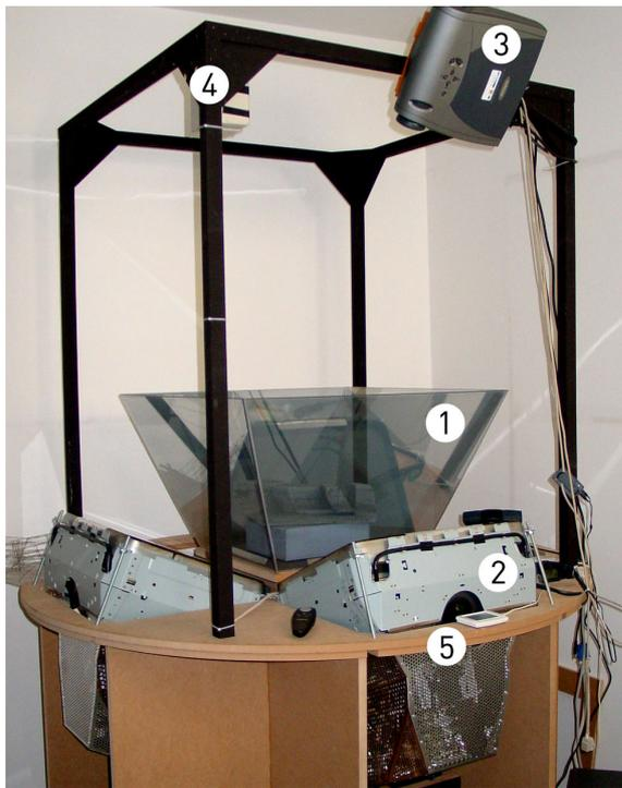
**Figure 1:** *The Virtual Showcase in our lab setup. The indicated parts are (1) half-silvered mirrors, (2) monitor for image generation, (3) light projector, (4) tracking system, (5) touch-pad for user interaction*
