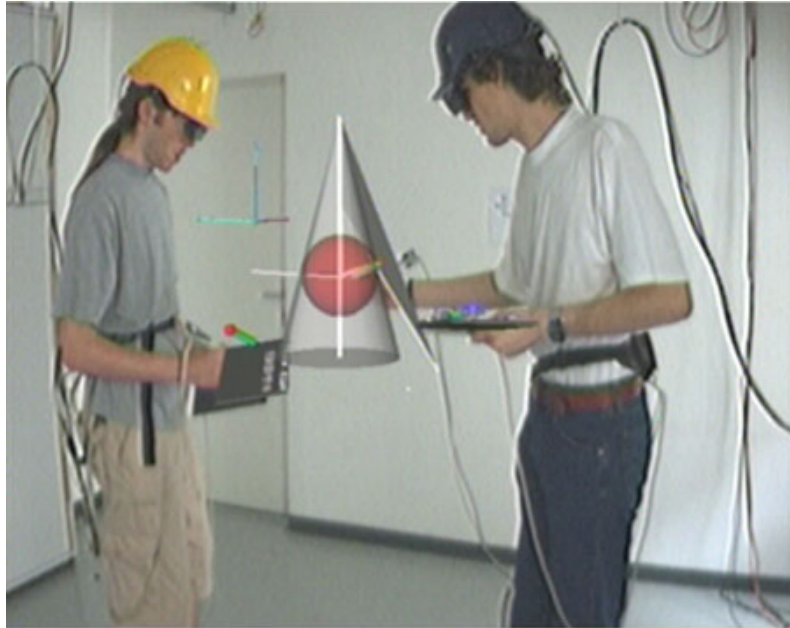
Figure 6: A typical Studierstube setup: two users collaborate in investigating virtual objects. The objects (cone and sphere in the center) are only visible through the HMDs the users are wearing. (Construct3D application setup, see [26])
