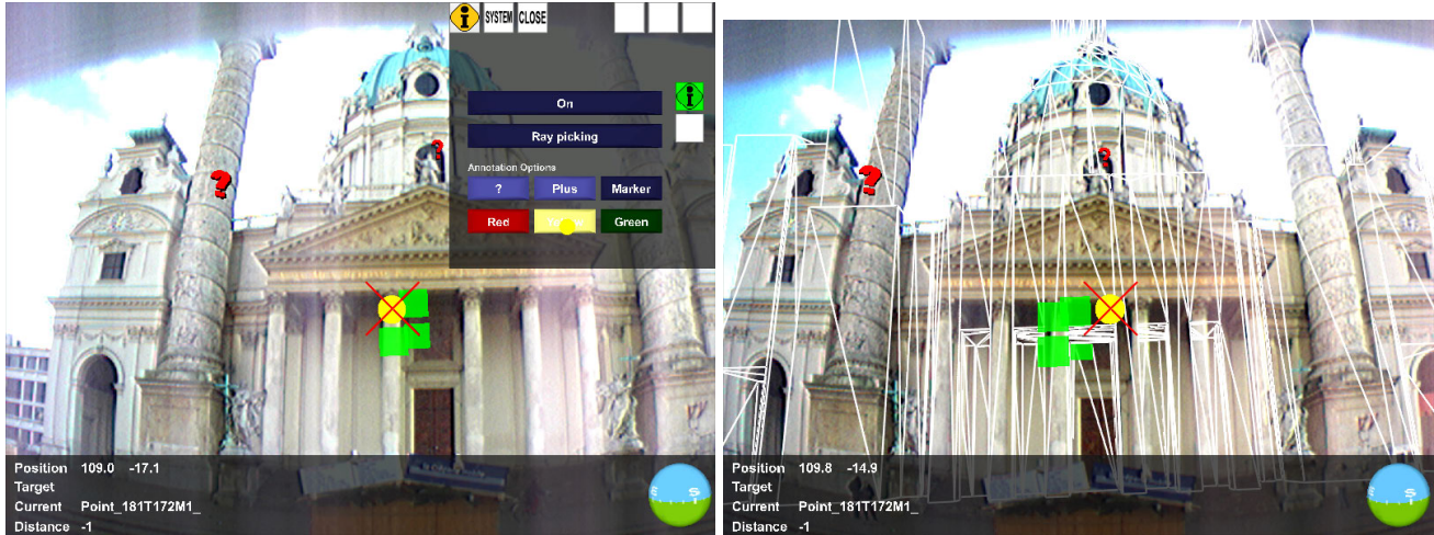
Figure 6. (Left) Annotation options and icons. (Right) The building geometry used for ray intersection is overlaid.
