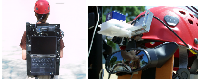
Figure 2. A laptop computer, GPS receiver and battery packs are mounted on a backpack. The HMD, inertial sensor and a camera are mounted on a helmet worn by the user.
