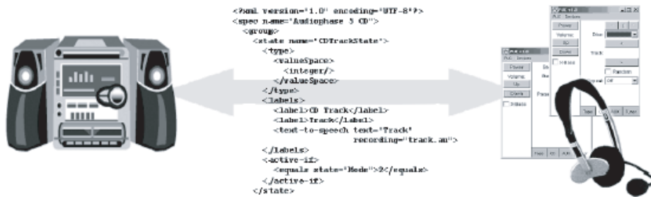
Figure 4: A diagrammatic overview of the PUC. A graphical or speech interface is introduced and communicates with the appliance by means of the specification language.
