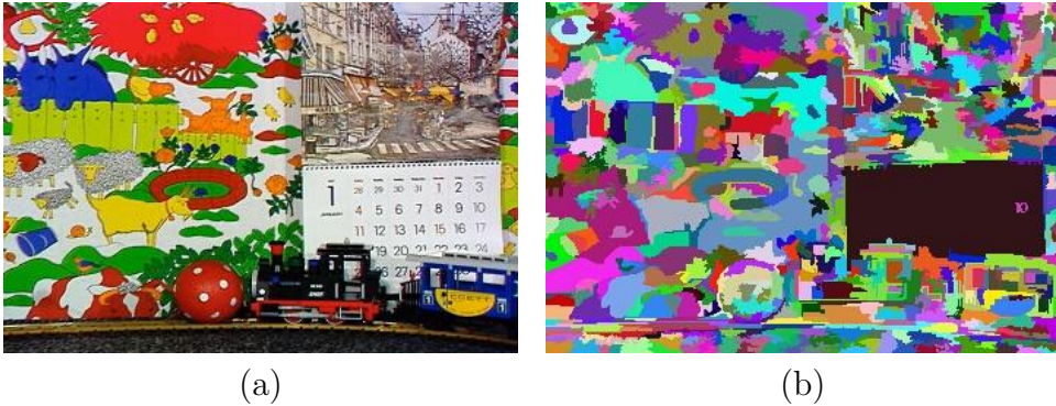
Figure 6.2: Colour segmentation. (a) Reference image. (b) Segmented image. Pixels of the same colour belong to the same segment.
