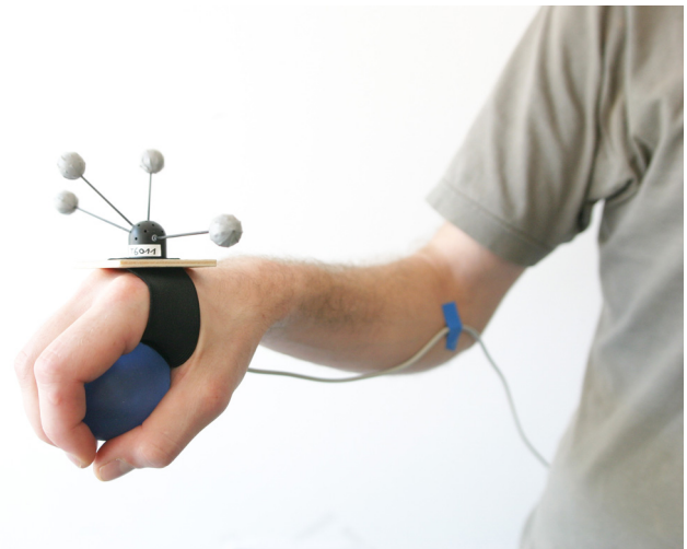
Figure 3: The SqueezeOrb can be combined with a rigid-body hand target for use as a general-purpose 6-DOF Analog Button.
