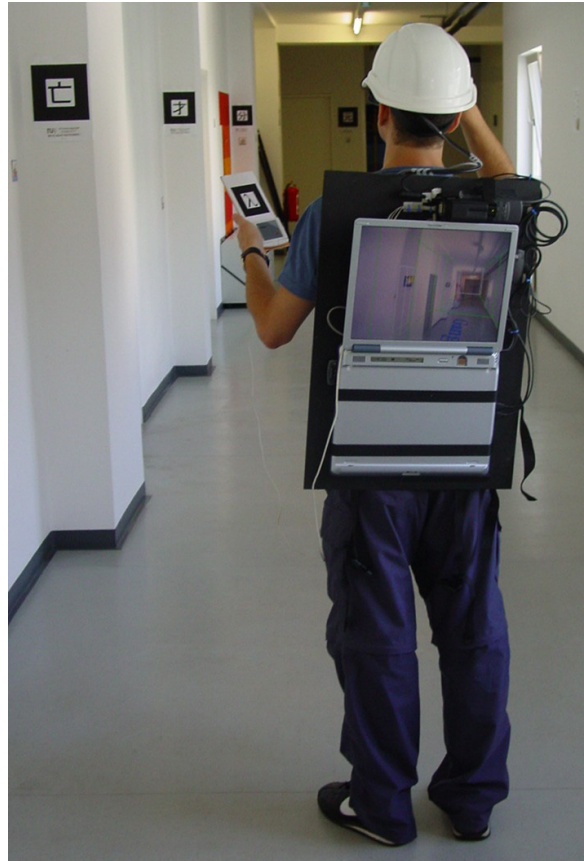
Figure 1. The user is guided through the building by the SignPost navigation system.
