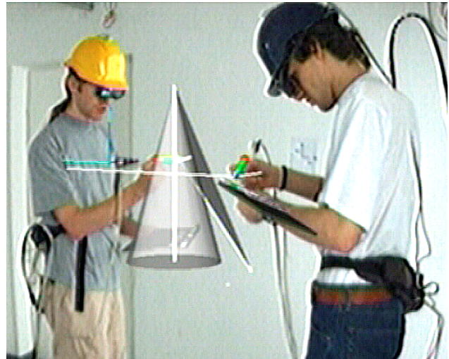
Figure 1: The distributed virtual workspace Studierstube supports multiple users and applications using tracked head mounted displays and hand-held tracked props. The image shows two users engaged in a geometry education task (live video overlay).
