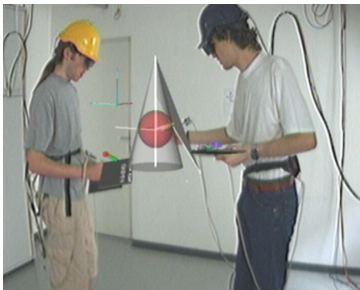
Figure 1. Students working with Construct3D in our lab. In this example they inscribe a sphere in a cone. The image is generated as live video capture with computer overlays.
