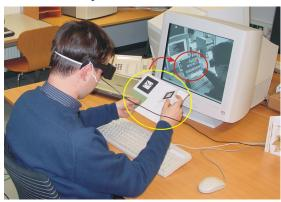
**Figure 4:** A user working with our desktop VR system. A FireWire camera (out of view) is used for optical tracking of the hand held props which are equipped with markers (see yellow ellipse). The image of the camera is used as a video background. Stereoscopic images are displayed on the monitor which give the user who wears shutter glasses the impression of working in 3D space. The virtual images of pen and PIP can be seen on the monitor (red ellipse) as an overlay over the video image.
