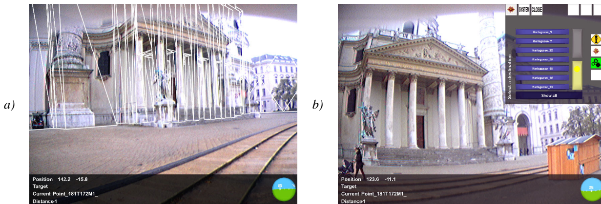
Figure 2. a) An overlay of the building model over the real world. b) 2D user interface components and HUD.
