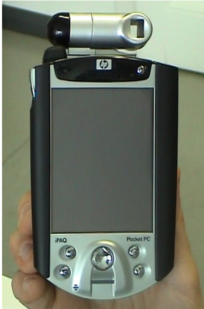
Figure 3. The IPAQ's CompactFlash camera is used for both optical tracking and as a source for the video see-through display
