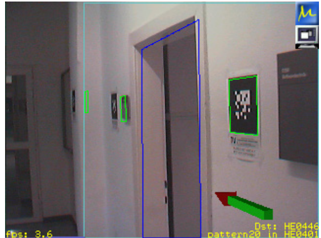
Figure 7. Signpost in stand-alone mode. Note the registered 3D overlays in the video image
