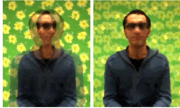
Figure 9: Adjusting the plane of zero parallax by horizontal image translation. On the left, the plane of zero parallax coincides with the background, while on the right the plane of zero parallax lies on the body of the subject.
