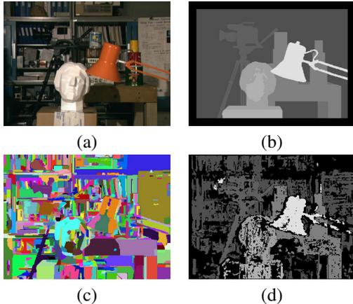
**Fig. 1.** Colour segmentation and initial disparity map. (a) Left image. (b) Ground truth provided with image pair. (c) Computed colour segmentation. (d) Computed initial disparity map. Invalid points are coloured black.
