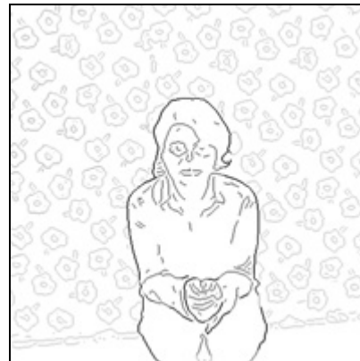
Figure 10: Edges extracted from the original image from Fig. 6 (a) with contour edges and foreground elements emphasized by darker gray values.
