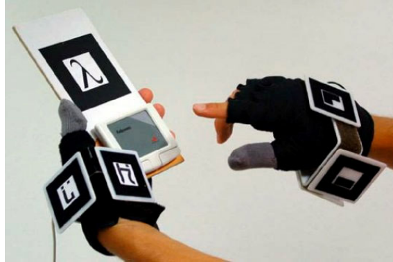
Figure 2.4: In this setup, ARToolkit markers are used to track the hands and an interaction device of the user.
