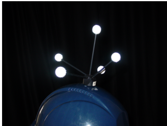
Figure 2.6: A target for the ART tracking system, composed of multiple retro-reflective balls. Note how the flashlight of the camera is reflected evenly from the surface of the balls.
