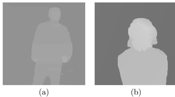
Figure 8. Disparity images on the geometry of the left view. (a) Disparity image for “Boy” dataset, (b) Disparity image for “Girl” dataset.
