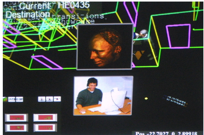
Figure 10: An indoor tour guide application, running on the desktop developer setup. A world-in-miniature view on the model of the building is shown in the background, and location-dependent HUD overlay graphics is presented to the user as she roams the building.
