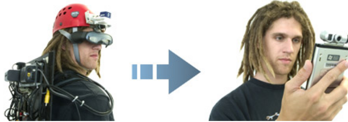
Figure 2: Evolution of mobile augmented reality systems. Early backpack-based systems (left) and our recent PDA-based handheld system (right).
