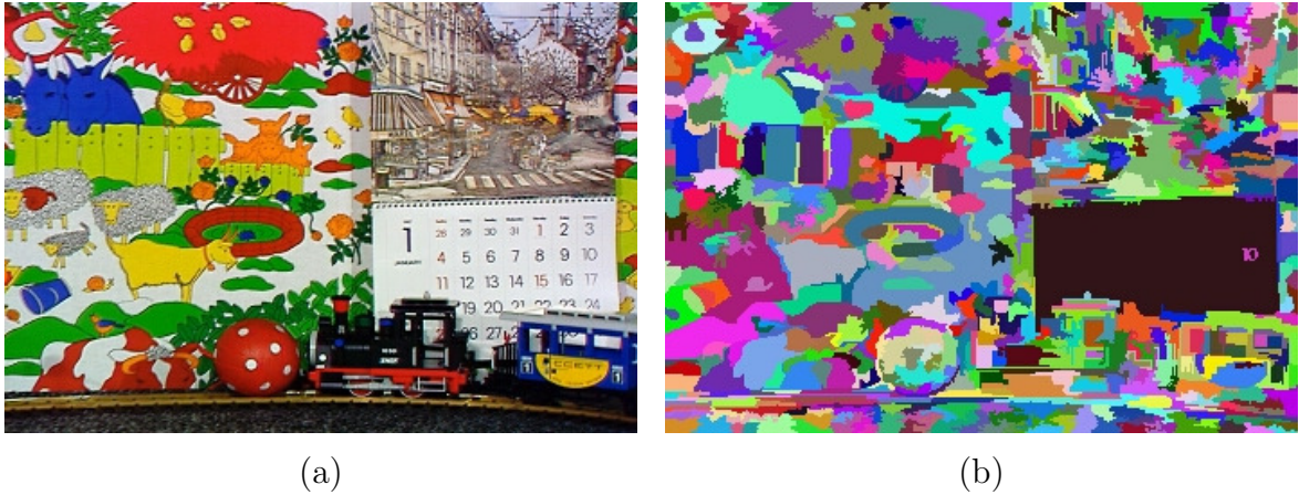
Figure 2: Colour segmentation. (a) Reference image. (b) Segmented image. Pixels of the same colour belong to the same segment.
