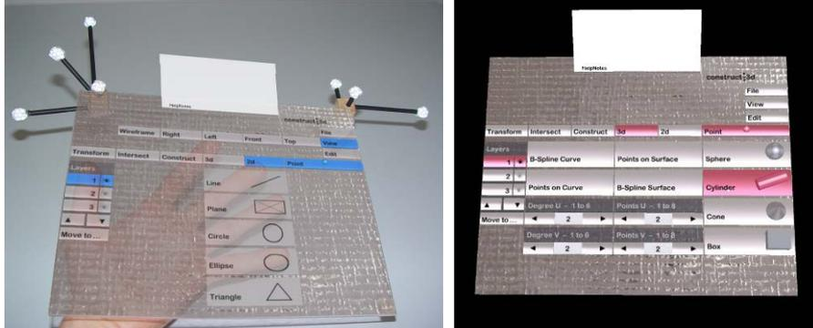
**Fig. 2.** Left: Menu system of Construct3D displayed on the PIP. In a help-box (on top) further details and help on application features are provided. Right: 3D submenu displayed for the user working with the red color scheme.
