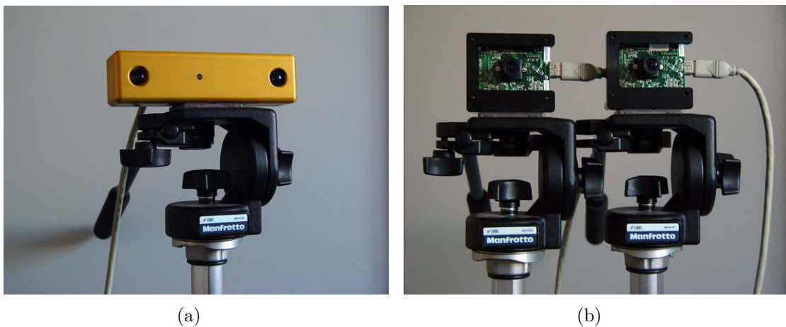
FIGURE 3.3 (a) PointGrey's Bumblebee , a commercially available stereoscopic camera, (b) stereo rig using two PointGrey DragonFly cameras .
