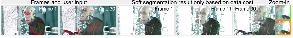
Figure 5.15: Video object segmentation based only on data cost (no smoothing). Left: Frames with red foreground scribbles. Right: Soft segmentation result. The zoom-ins show the results before ( bottom ) and after ( top ) alpha matting. Copyright of original video: Blender Foundation.
