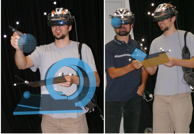
Figure 2: Left: A student working with PhysicsPlayground. In the right hand he holds a wireless pen (used as input device), in the left hand the PIP. Right: Collaborative work in PhysicsPlayground.
