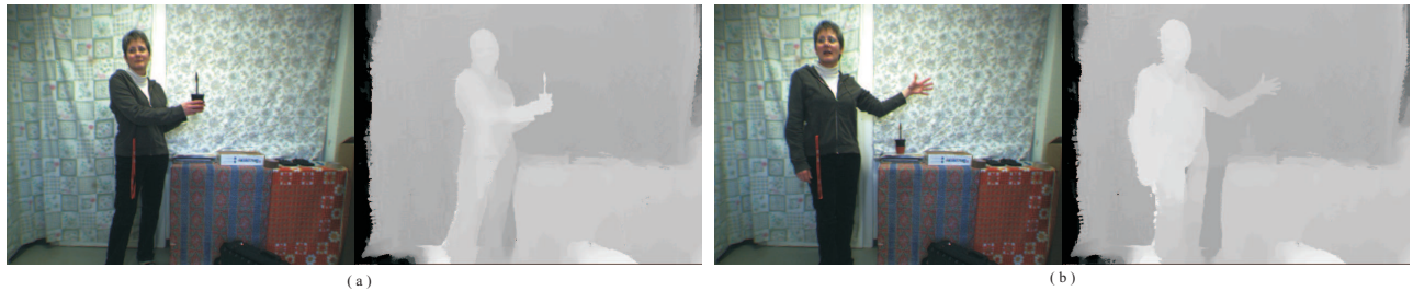
Fig. 4. Two sample frames captured by our live system and their corresponding disparity maps. (a) Shot 1 (b) Shot 2.
